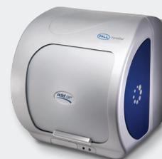
The Octet QK<sup>e</sup> system is the enhanced-performance version of the first-generation Octet QK instrument from the Octet family of label-free biomolecular interaction analysis instruments. Two acquisition rate settings and a higher-performance spectrometer combine to provide greater sensitivity and a wider dynamic range for protein quantitation and kinetic analysis. In addition, biosensor re-racking provides enhanced assay flexibility and operational cost savings.
