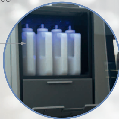
Easily access wash bottles, washer and waste from front of instrument
