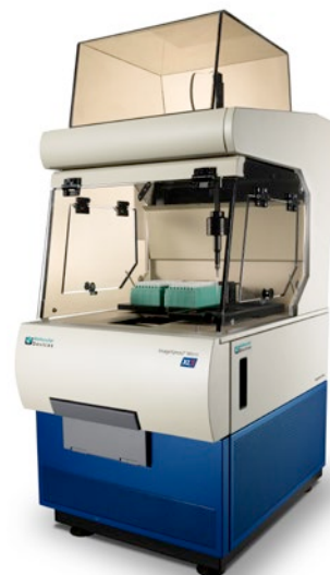
ImageXpress Micro XLS System with Fluidics Option installed.
