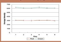
The GenePix 4000B Scanner offers proven repeatability, scan after scan. A non-bleaching fluorescent test standard was scanned repeatedly and the average signal was quantified. Signal value variance among all scans was 1.6% in the green channel and 2.1% in the red channel. Error bars cover two SD from the mean of the four measurements at each time point.
