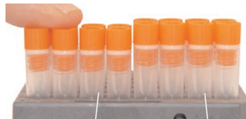
TubeLock activated, tubes locked into position
