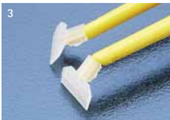
3 The blade of the cell scraper is made of soft material; this protects the cells.
